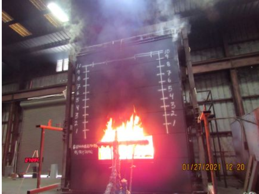
Photo No. 26 Flame height at 2 ft above window
