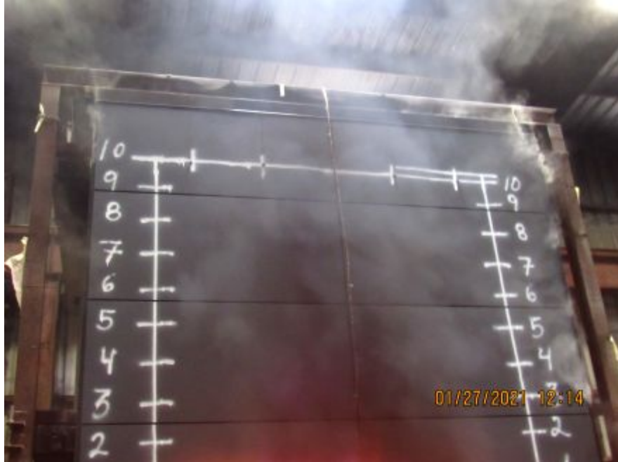
Photo No. 24 Smoking from top of wall
