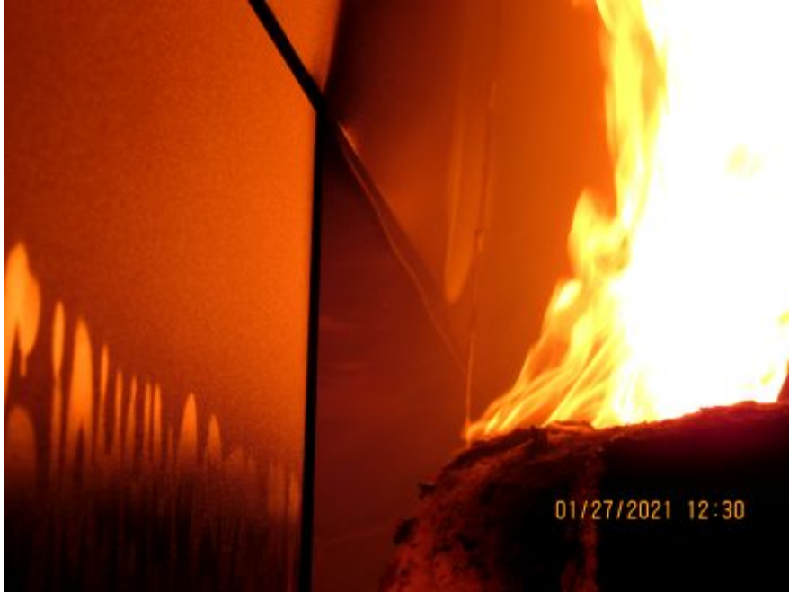
Photo No. 29 Panels opening up
