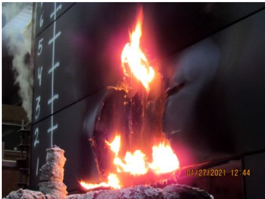
Photo No. 32 Residual flaming post-test
