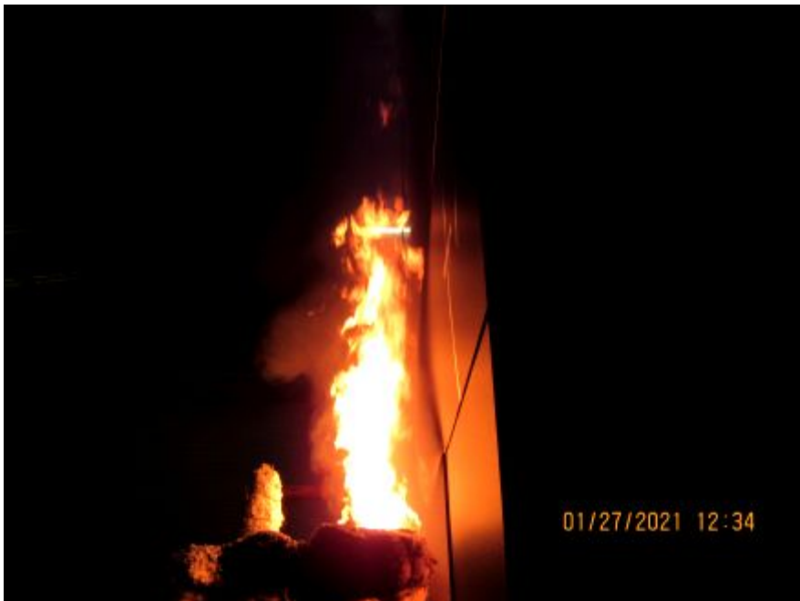
Photo No. 30 Second row panels opening up
